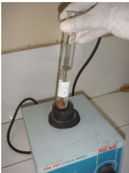
Figure 7. Agitation of tissue immersed in test solution with the help of cyclomixer
