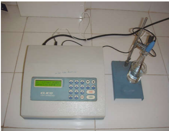
Figure 6. Measuring the pH of the solutions sample
