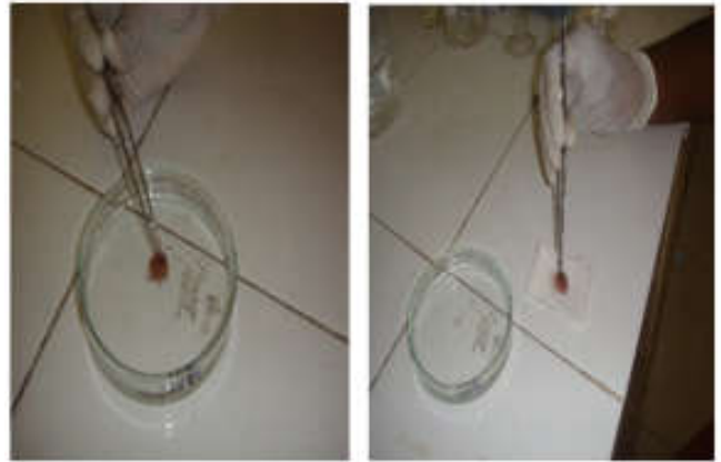
Figure 8. Submersion in distilled water and blotting dry of sample
