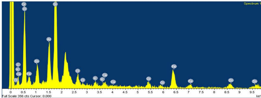
**Fig. 2. EDX of the Electroplating effluent contaminated soil**
