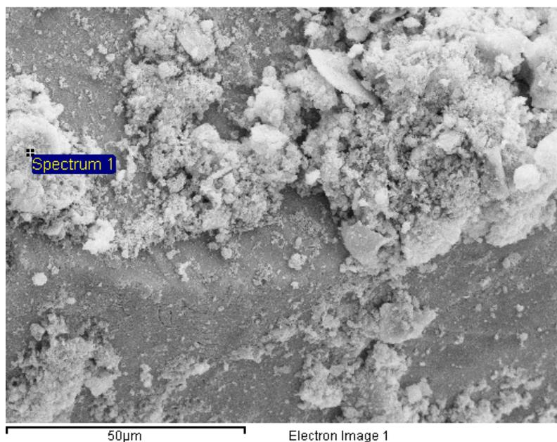
**Fig. 1. SEM-EDX of the Electroplating effluent contaminated soil**
