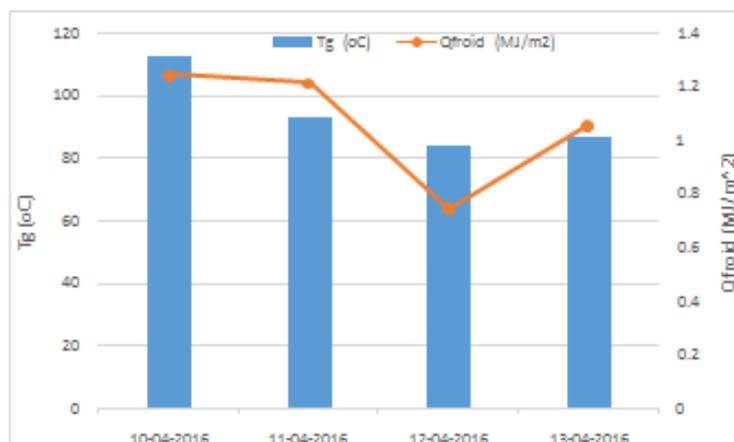
Figure 11. Influence of the regeneration temperature on the amount of cold produced
