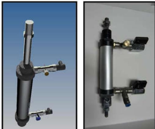
Figure 8. Pneumatic System Double Acting Cylinder
