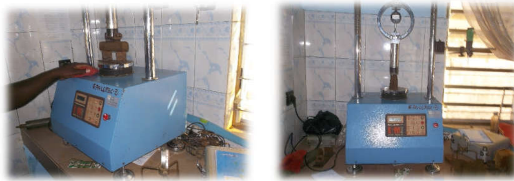
Figure 5. Compressive and flexion strengths device
