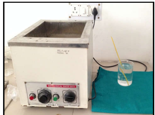
Fig. 5. Thermocycling of samples
