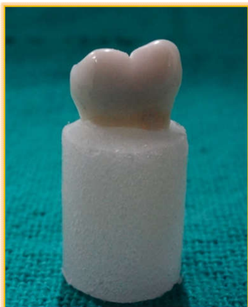
Fig. 3. Each half embedded in autopolymerizing acrylic resin
