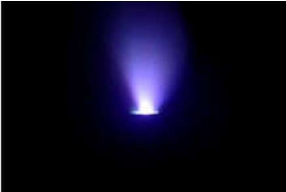
Image1 credit: NASA images Pulsed Plasma Thruster in operation
