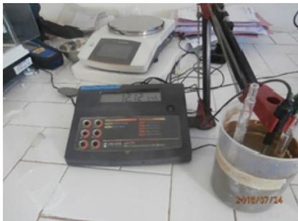
Photo 1. Liming of sludge at pH = 12
