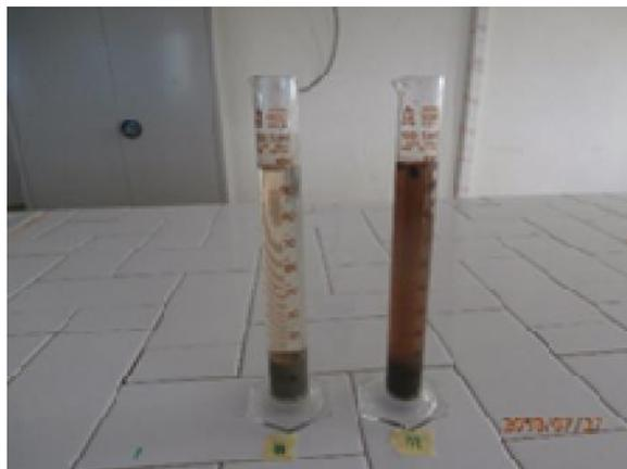
Photo 3. Test of settling of stabilized sludge with test-tube
