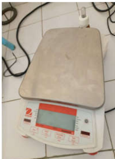
Figure 2. balance with precision of 0.001g
