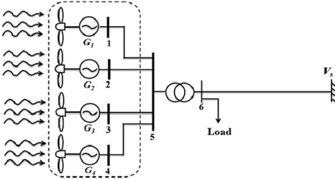
Fig.1 Multimachine marine turbine system connected to infinite bus
