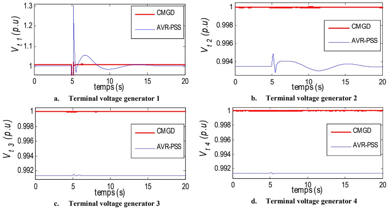
Fig. 3. Generators terminal voltage for a short-circuit of 200ms duration after 5s
