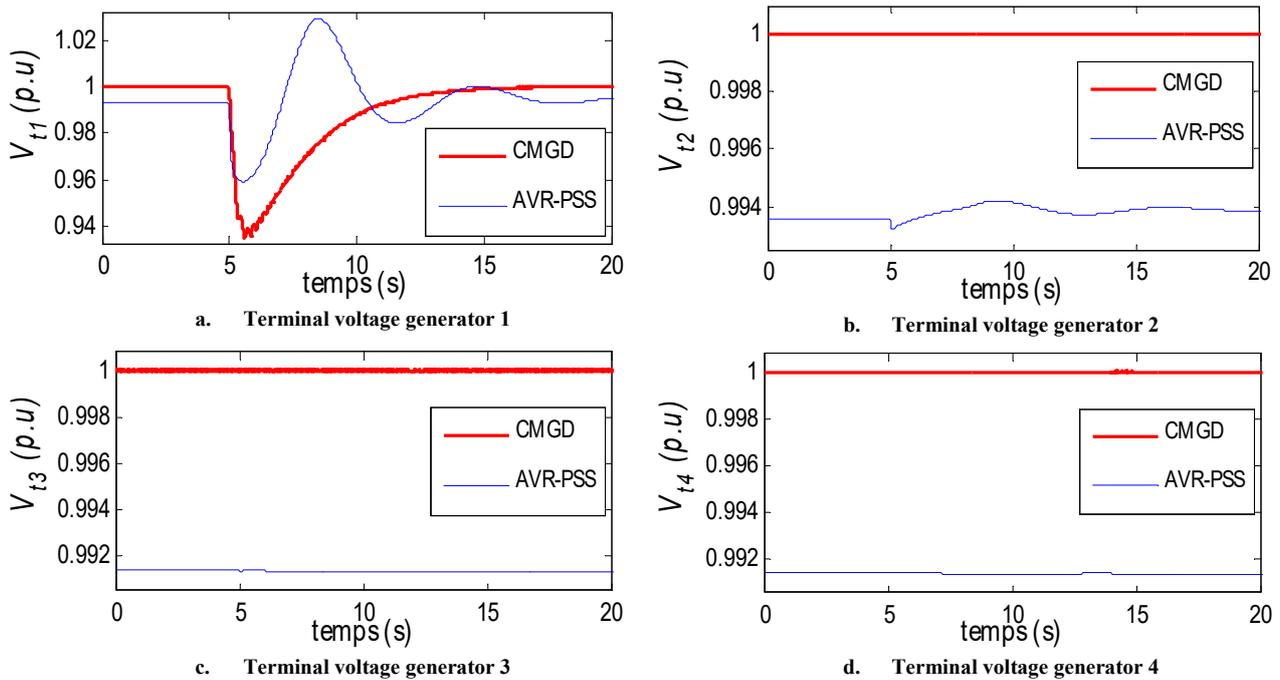
Fig. 5. Generators terminal voltage for mechanical power drop of 50% of its value
