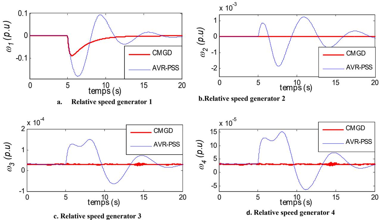
Fig.4. Generators relative speed for mechanical power drop of 50% of its value
