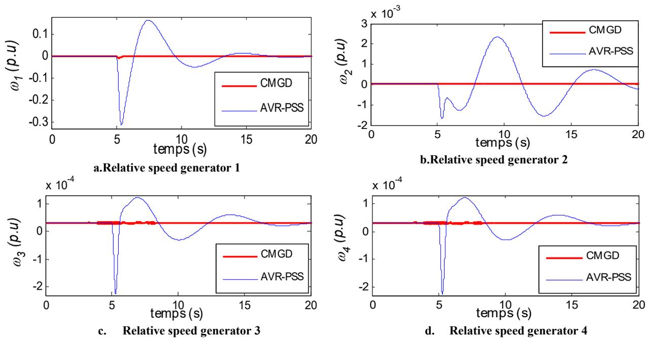
Fig. 2. Generators relative speed for a short-circuit of 200ms duration after 5s
