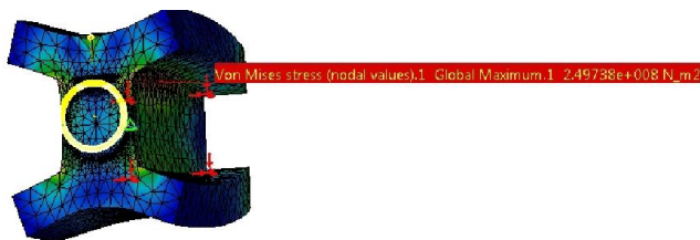
Fig. 7. Von Mises Stress Distribution of I-Beam
