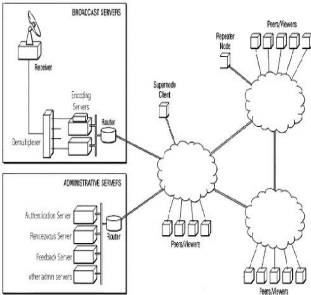
Although a peer can freely switch from one TV channel to another, thereby departing and joining different peer-to-peer networks, it can only join one peer-to-peer network at any one time. We henceforth limit our description of the Zattoo delivery network as it pertains to carrying one TV channel. Fig. 1 shows a typical setup of a single TV channel carried on the Zattoo network.
