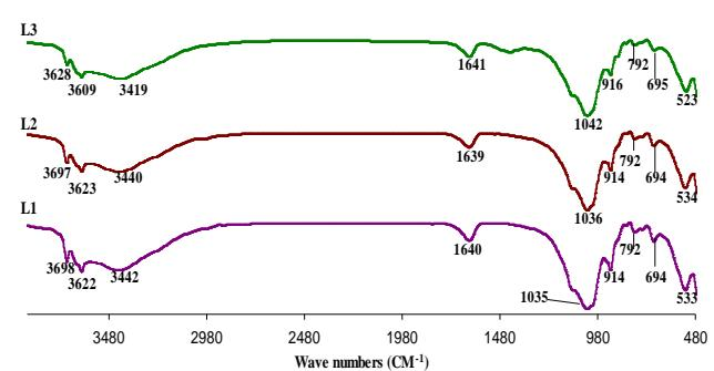
**Figure 3.** FTIR for untreated samples L<sub>1</sub>, L<sub>2</sub> and L<sub>3</sub>
