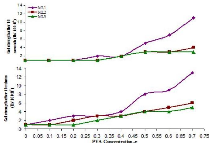
Figure 8. G<sub>10sec</sub>, G<sub>10 min</sub>, and concentration of PVA relationship of formulated muds (ML<sub>1</sub>, ML<sub>2</sub> and ML<sub>3</sub>)
