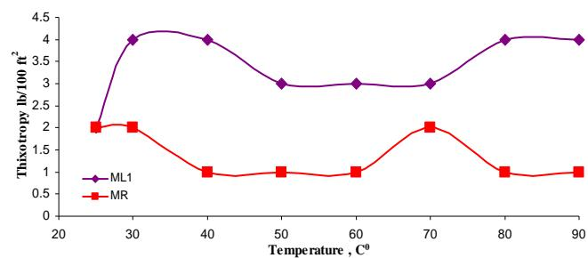
**Figure 12. Temperature relationship, Thixotropy of formulated mud ML<sub>1</sub> compared to MR**
