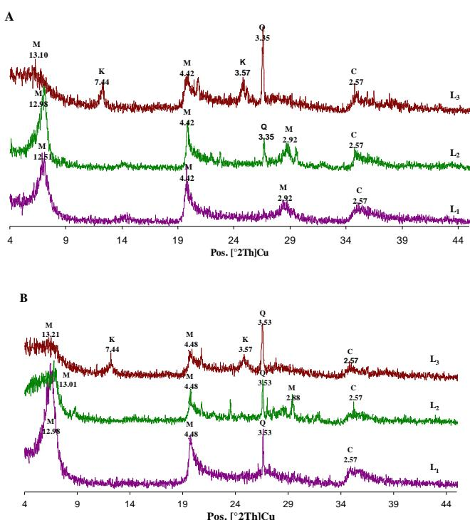
**Figure 1. (A) X-ray diffraction analysis of untreated samples (L<sub>1</sub>, L<sub>2</sub> and L<sub>3</sub>) and (B) for treated bentonite samples (L<sub>1</sub>, L<sub>2</sub> and L<sub>3</sub>) with PVA( M=Montmorillonite, C= Calsite, K= Kaolinite and Q= Quartz)**
