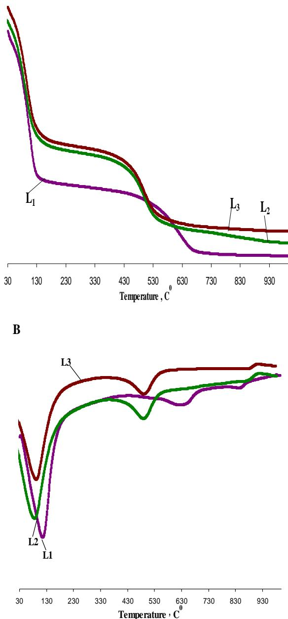
**Figure 2.** TGA for Fig. (A) and DTA for Fig. (B) For local untreated bentonite samples L<sub>1</sub>, L<sub>2</sub> and L<sub>3</sub>
