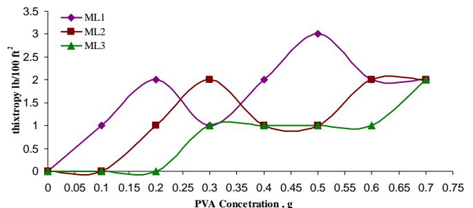
Figure 9. Concentration of PVA and Thixotropy of formulated muds (ML<sub>1</sub>, ML<sub>2</sub> and ML<sub>3</sub>)
