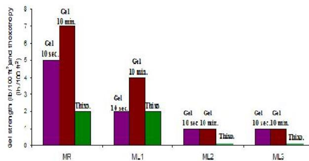
**Fig 6. Gel strength after 10 sec. and after 10 min. and thixotrop for  $ML_1$ ,  $ML_2$  and  $ML_3$  before activation with PVA compared with MR**
