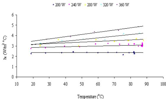
**Fig. 2:  $h_c$  Vs Temperature at different rate of heat inputs for stainless steel pot**
