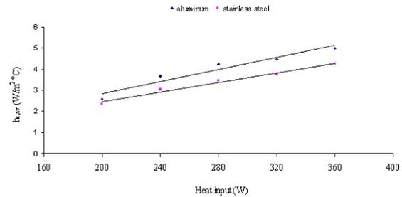
**Fig. 4:  $h$  Vs heat inputs for stainless steel and an aluminum pot**
