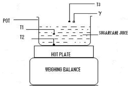
Fig. 1. Schematic view of experimental unit
