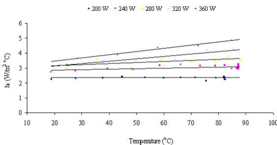
**Fig. 3:  $h_c$  Vs Temperature at different rate of heat inputs for an aluminum pot**
