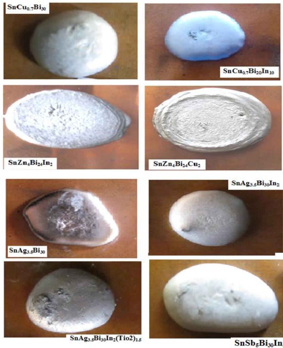
Figure 4. Photo graphs for tin- bismuth based alloys spreading on copper substrate in air
