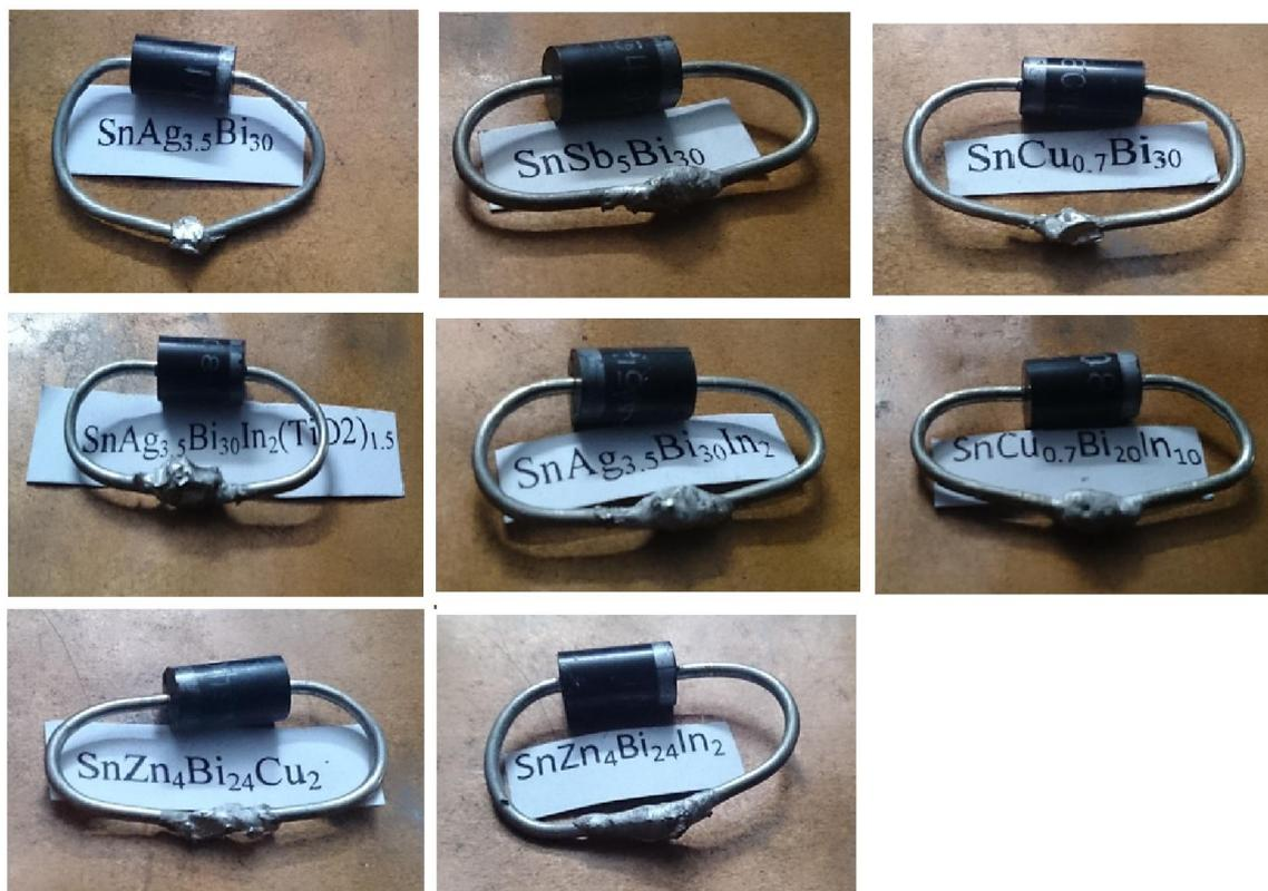
Figure 5. Photo graphs for soldering process of tin- bismuth based alloys in electronic devices
