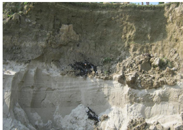
Plate IV: Unconsolidated sand at bottom and thin silt clay soil at top at Mithipur area
