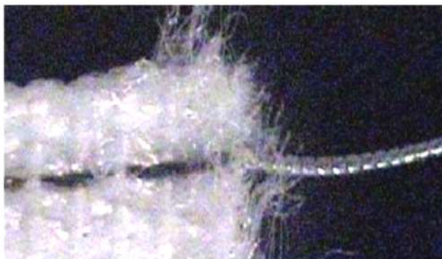
Figure 8. Interwoven Specialty Core Optical Fibers/Sheath Cotton/Polyester Yarns Wire –Sheath Fibers Yarns
