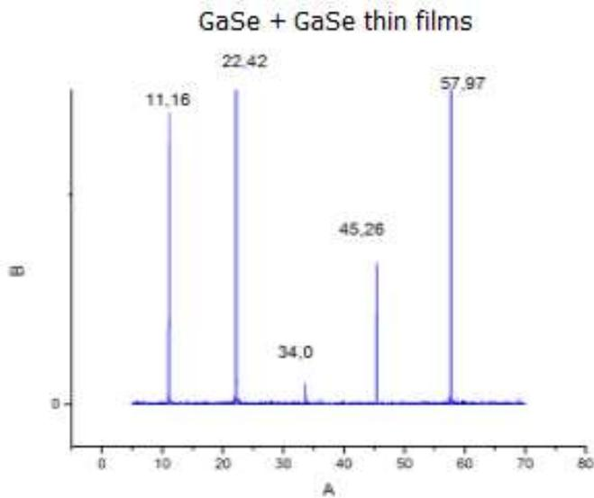
Fig. 2. Diffraction pattern (XRD) for GaSe nanoparticles on GaSe substrate
