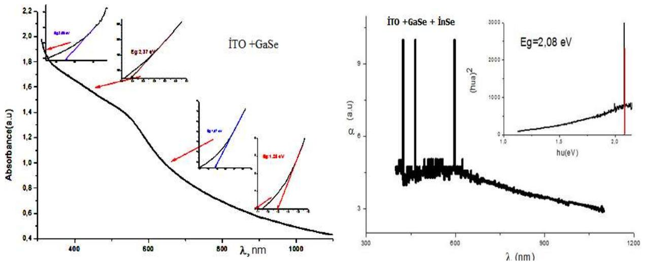
Fig. 8. a) Absorption spectrum of GaSe nanoparticles on a glass substrate, b) Absorption spectrum of ITO + GaSe + InSe
