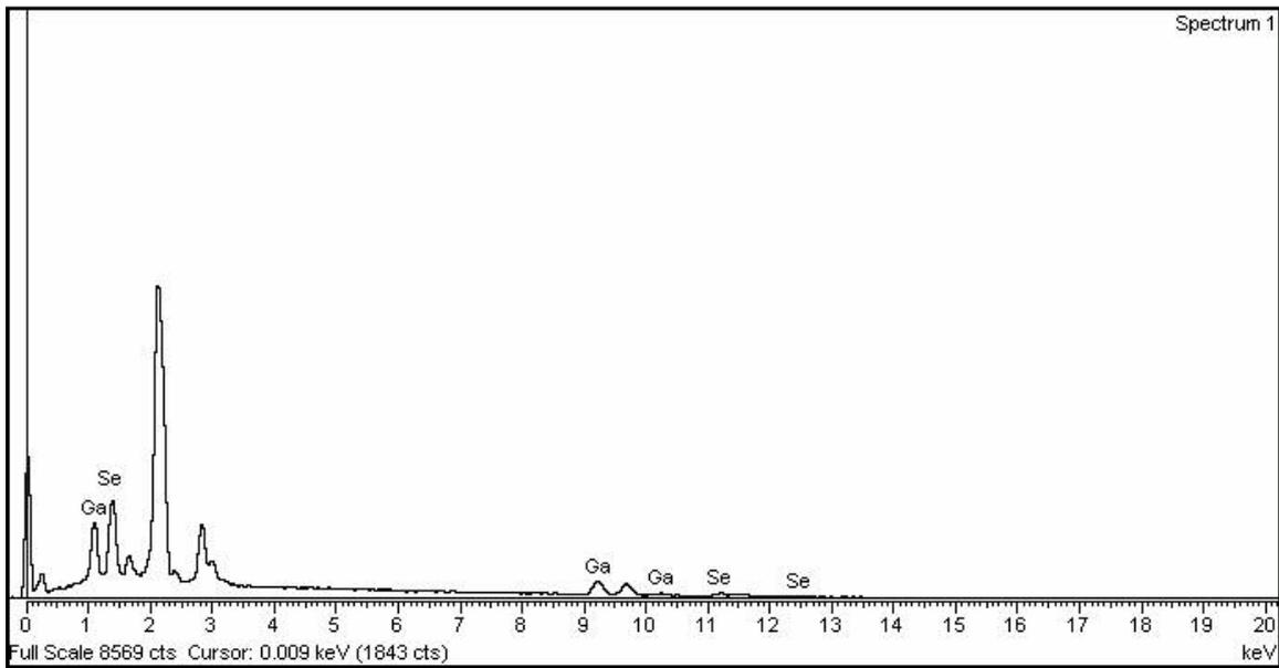
Fig. 4. EDAX images for GaSe nano-particles
