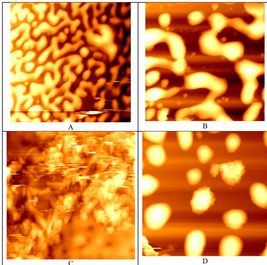
Fig. 3. AFM images of GaSe nano-particles on a glass substrate (a), (b) and on GaSe substrate (c), (d) before (a, c) and after (c, d) annealing, accordingly
