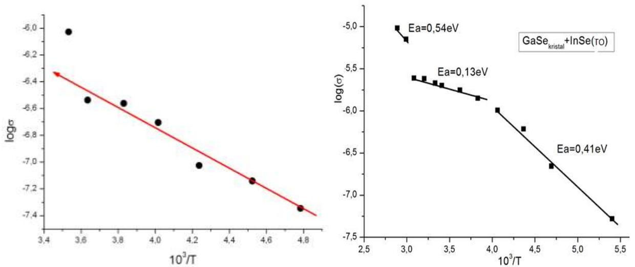
Fig. 6.  $\log \sigma = f(1/T)$  for GaSe + GaSe (a) and for GaSe + InSe (b)
