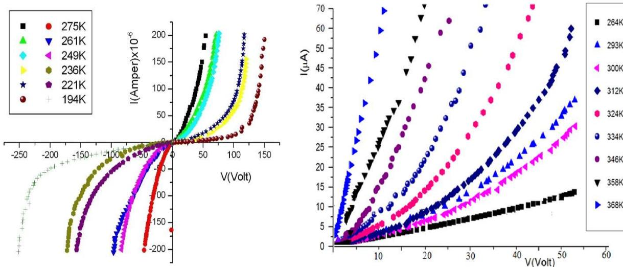
Fig. 7. Current-voltage characteristics of GaSe (a) and InSe(b) nanoparticles on GaSe substrate at different temperatures
