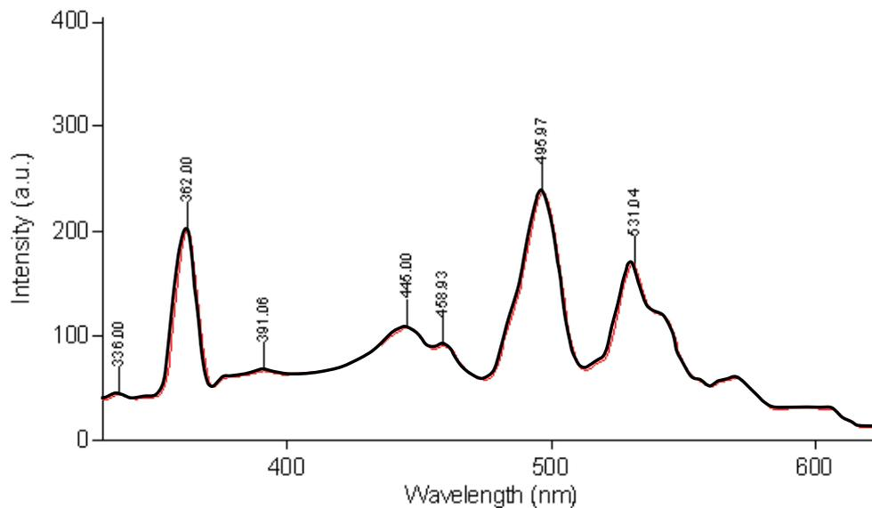
Fig. 9. Photoluminescence spectra of GaSe nanoparticles on a glass substrate
