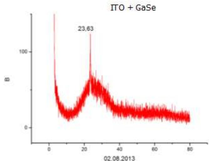
Fig. 1. Diffraction pattern (XRD) for GaSe nanoparticles on a glass substrate
