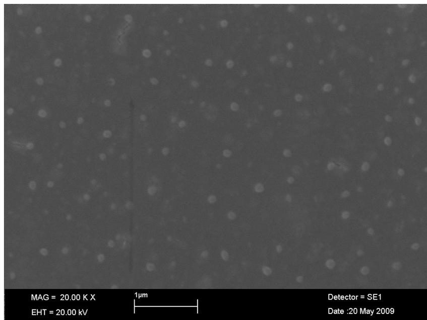
Fig. 5. SEM image for GaSe on a glass
