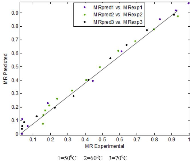
Fig. 5. Comparison of experimental and predicted moisture ratio with time at different temperatures using Page model
