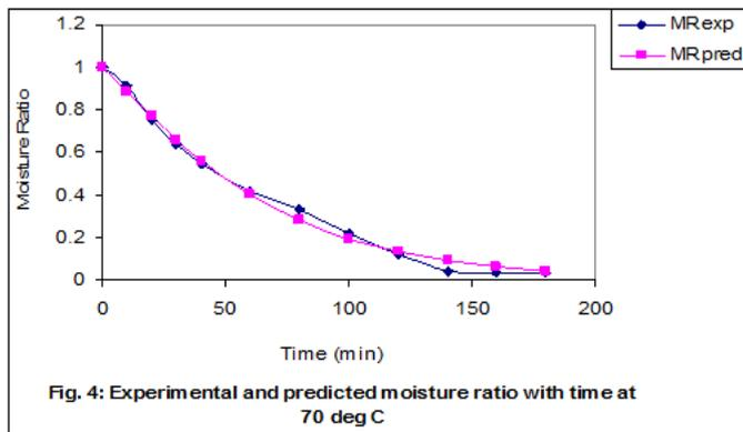
Fig. 4: Experimental and predicted moisture ratio with time at 70 deg C
