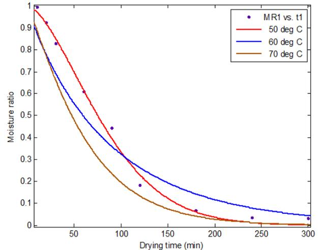
**Fig. 1. Variation of moisture ratio with time at different drying temperatures (using Page model)**
