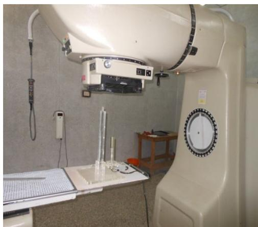
Fig 2. Mini-phantom experimental set-up for  $S_c$  measurement
