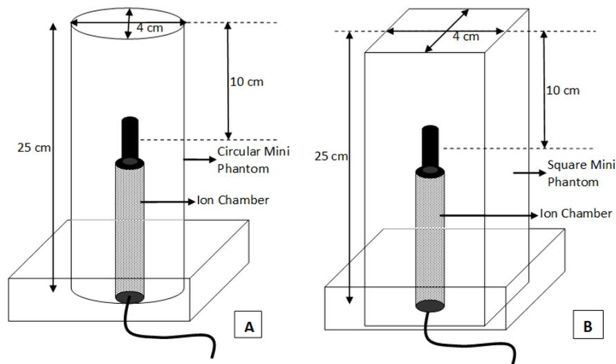
Fig 1. Block diagram of circular and square mini-phantoms
