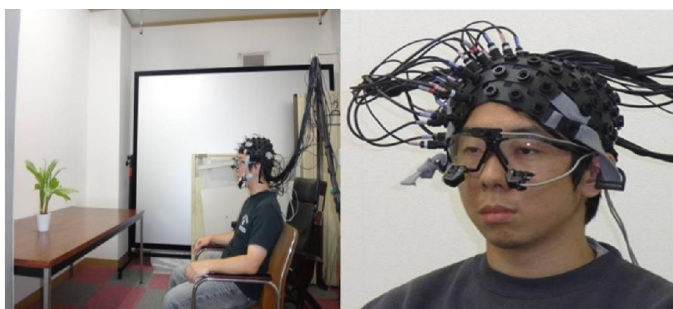
Fig. 2. Experimental setting and physiological measures, eye mark recorder and multi channel near infrared spectroscopy
